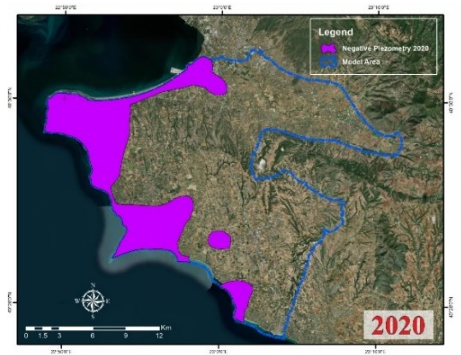
Figure 3.5 Zones with negative piezometric head in Eastern Thermaikos Gulf and Anthemountas basin for the year 2020.
