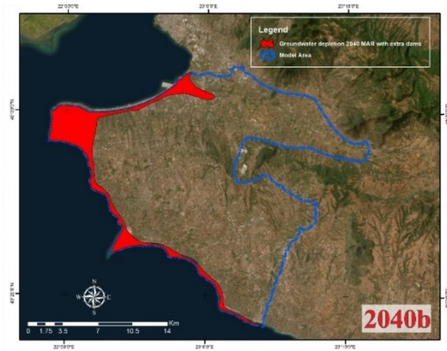
Figure 3.4 Groundwater depletion zones in Eastern Thermaikos Gulf and Anthemountas basin for the year 2040 applying scenario B (MAR application with extra dams).
