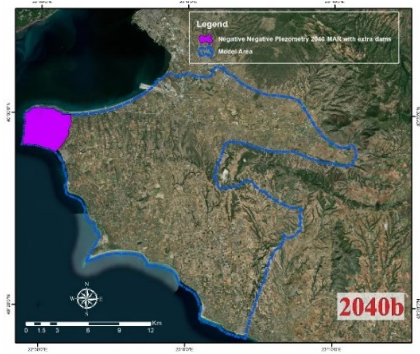
Figure 3.8 Zones with negative piezometric head in Eastern Thermaikos Gulf and Anthemountas basin for the year 2040 applying scenario B (MAR application with extra dams).
