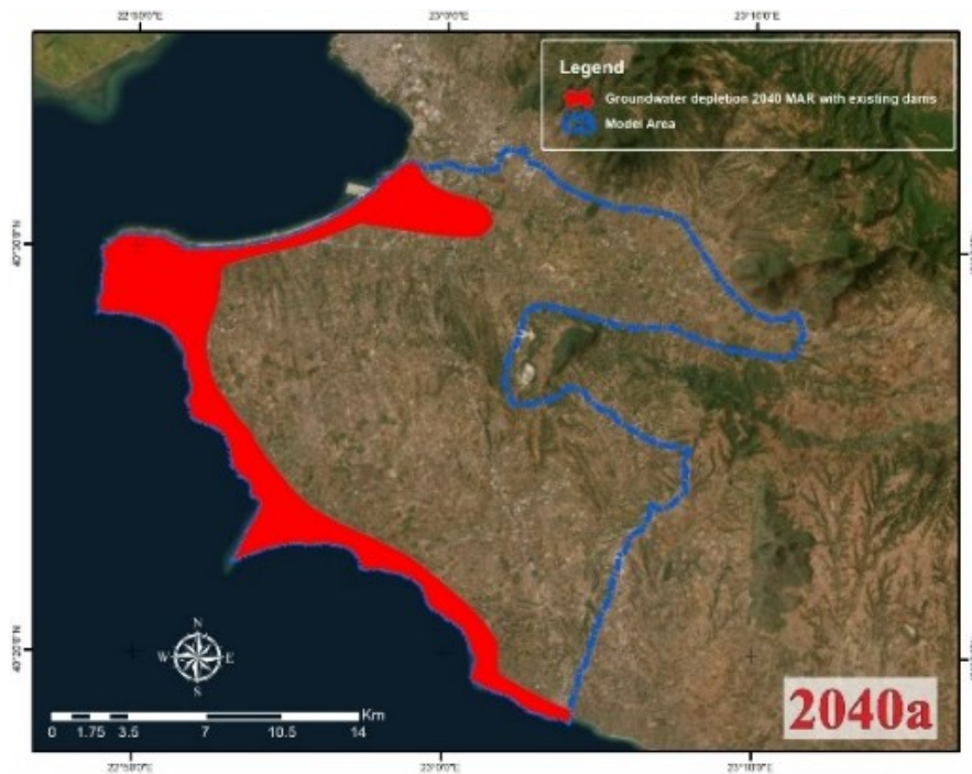
Figure 3.3 Groundwater depletion zones in Eastern Thermaikos Gulf and Anthemountas basin for the year 2040 applying scenario A (MAR application with existing dams).
