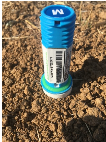
Figure 5.16 Probe for soil moisture and temperature.
