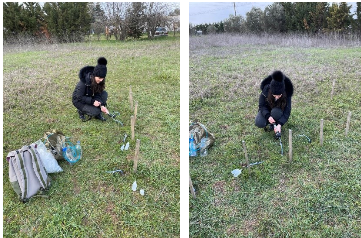
Figure 5.13 Process to collect water from the ceramic cups.
